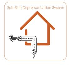
slab or using vertical pipes that extract through the slab, and using a fan to "suck" out and blow the contaminated air away from, rather than into, the building's interior. This is called a sub-slab depressurization system (SSDS) or a sub-slab ventilation system.
